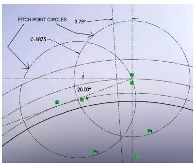
8. Now draw a 3 Point Arc from the intersection of the Outside Diameter to the Pitch Diameter with the third point on the second Pitch Point Circle. Refer to the image nearby.
