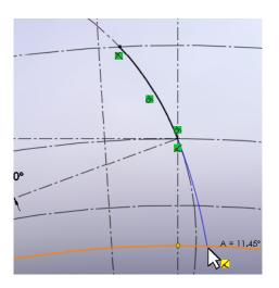
10. To make the last arc sketched perpendicular to the Root Diameter, sketch a Construction Line from the endpoint of the arc sketched above to the Origin. Make this line tangent to the arc sketched above. For some of the designs this arc will almost be Coradial with the second Pitch Point Circle but not always.
