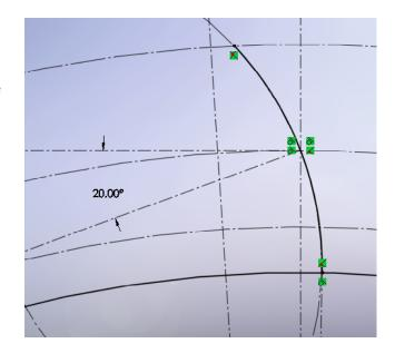
11. Now mirror the two arcs sketched above using the line representing half of the angular Circular Thickness. Sketch a 3 Point Arc connecting the two endpoints of the mirrored arcs on top with the third point on the Outside Diameter. You should now have 2 areas of enclosed geometry ready for some 3D features.
