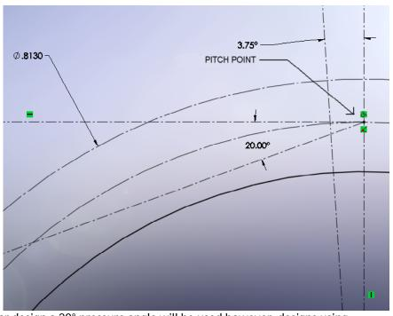
rotating clockwise. In our gear design a 20° pressure angle will be used however, designs using other angles, such as 14.5° are less common but can also be found. The sketch now should look similar to the image nearby.
