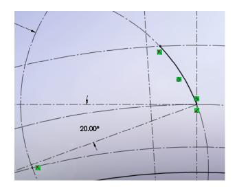
9. Sketch a Tangent Arc from the bottom end point of the 3 Point Arc sketched above to the Root Diameter. Refer to the image nearby.
