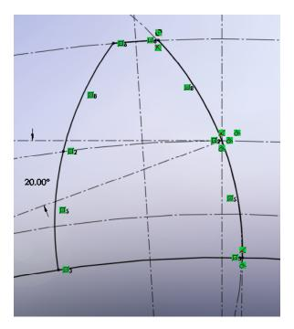
12. Go to the "Extrude Boss/Base" and extrude using the Mid Plane direction option, a distance of your choice, selecting the center region of the gear in the "Selected Contours" section of the Properties Manager. Name this feature "Base Extrude". Borrow the sketch from the first feature and using the "Extrude Boss/Base" feature again extrude the region for the gear tooth a distance less than the first extrude. Name this feature "Gear Tooth".
